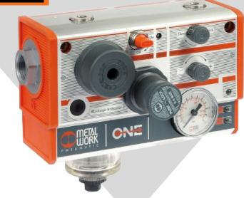
One single unit houses the threaded ports, filter, condensation drain, pressure regulator, shut-off valve, soft start valve, pressure switch and three supplementary air intakes.
