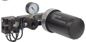
Vaccon's Mid Series venturi vacuum pumps with Air-Saver-Technology are all pneumatic systems that minimizes compressed air usage by creating, monitoring and maintaining vacuum for safe energy efficient operations. When the desired vacuum setpoint is reached, the air supply is isolated, saving compressed air. If the vacuum level drops by 3" Hg, the air supply is re-engaged to restore the necessary vacuum.
