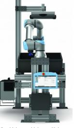
Most machine tending applications can be automated with the robot. We will deliver you a complete custom collaborative robot machine tending kit by combining multiple components with application-specific hardware and software to get closer to your solution.
